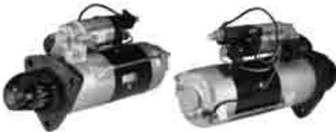
2-2773-ND (Ref# 18571N) Starter - Nippondenso PLGR 5.0kW/12 Volt, CW, 12-Tooth Pinion
