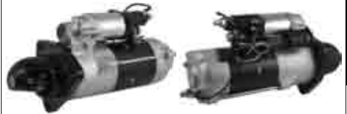
2-2886-ND (Ref# 18577N) Starter - Nippondenso PLGR 8.0kW/24 Volt, CW, 12-Tooth Pinion
