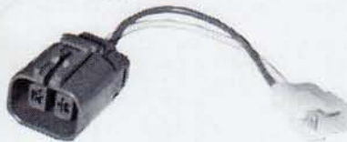
Converts "SL" oval plug to "T" shaped alternator plug
