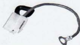
Convert "T" shaped S & L into 1 wire alternators
