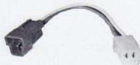
Early 3 wire Toyota to early 2 wire Datsun conversion harness
